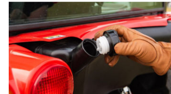
5. High-capacity fuel tank
