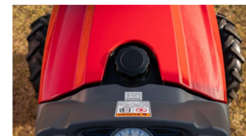
6. Large-volume fuel tank
