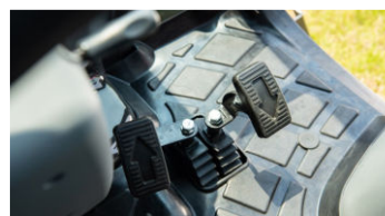
4. Highly responsive forward & reverse HST (T4048 (5025CH))
