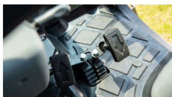
4. Highly responsive forward & reverse HST (T4058 (6225CH))
