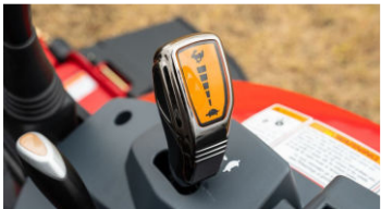
1. 2 range hydrostatic transmission (HST)
